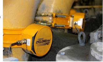
The CYCLONEtrac PST system consists of individual sensor assemblies mounted to hydrocyclone overflow pipes, junction boxes, and a control room computer. The sensor assembly is made up of a ruggedized probe that is in contact with the overflow stream and an integrated electronics package that is protected by a sealed metal enclosure. The sensor assembly is wired to the junction boxes located near the hydrocyclone battery. The junction box receives 100-240 VAC power and supplies
