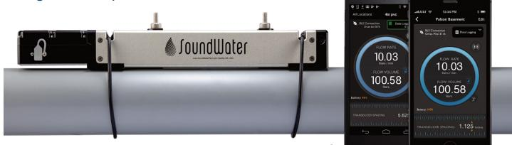
**Orcas** is a portable ultrasonic flowmeter designed for speed and ease of use. With the Orcas, you can capture accurate and reliable flow measurements in under one minute—saving you time and money.
